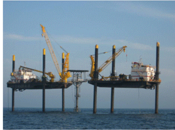
200-ft. class Superior Intervention and Superior Excellence supporting well intervention project (coiled tubing/nitrogen stimulation and electric line) in 72-ft. of water in GOM
